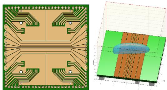
*Figure 1 - PCB (left) has current carrying wire structure capable of producing a trapping magnetic potential for the atoms. Simulation (right) shows the resulting shape of the trapped atomic cloud (blue).*
