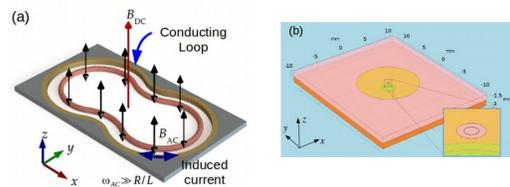
**Figure 1.** (a) Schematic of the working principle of a MW-dressed ring trap for cold atoms (b) Design of an atomchip realization of the ring trap.
