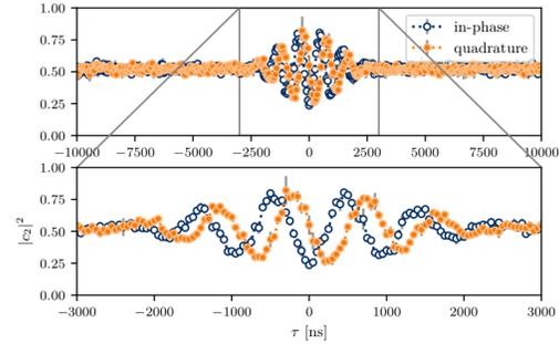
Figure 2: Quadrature interferometer signal measured as a function of  $\tau$ , the temporal asymmetry introduced to the pulse sequence.
