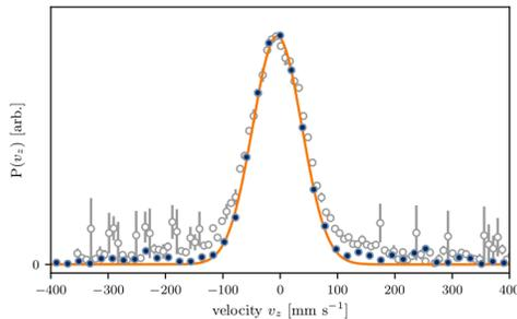
Figure 1: Interferometric measurement of a velocity distribution (filled circles) to which a Gaussian is fitted (solid line) corresponding to a temperature of  $17\mu\text{K}$ . Doppler Raman spectroscopy data are also shown (empty circles), revealing differences in the wings.
