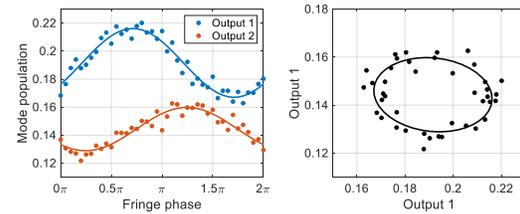
Figure 1: Measurement of two interferometer outputs with  $\pi/2$  phase shift between them, shown each vs. absolute fringe phase (left) and each vs. the other (right).
