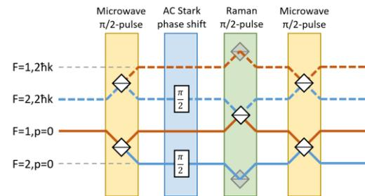
Figure 2: Our composite beam splitter, which creates four quadrature output signals in four atomic states, separated in momentum and internal state.
